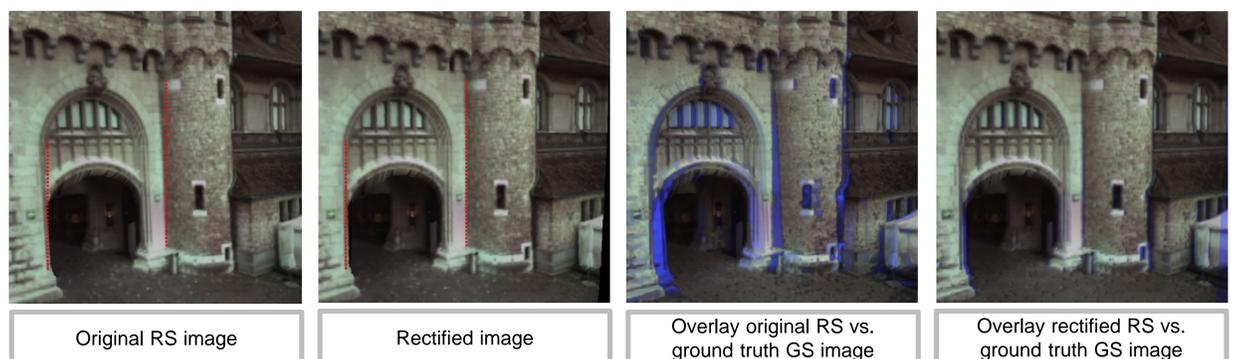
Fig. 4: The above "castle" images were rendered using [5] based on a 3D model provided by [6]. Overlay deviation is shown in blue.
