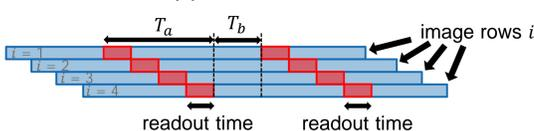
Fig. 2: Shows how the pixels of a RS camera are recorded. The image rows are taken sequentially.
